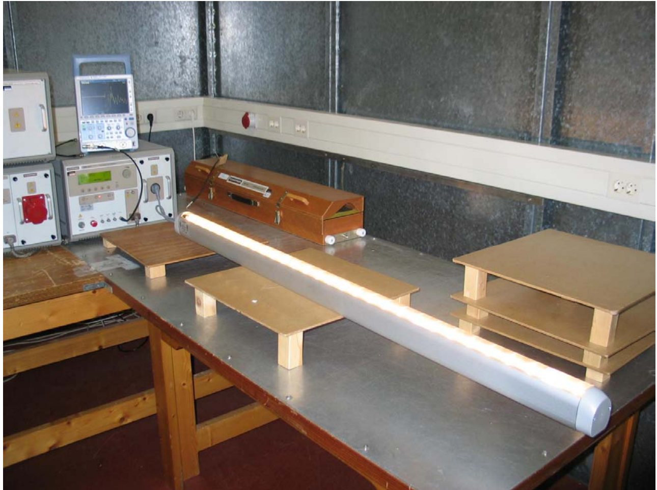
Photo 7. Basic setup for EFT Immunity Testing
