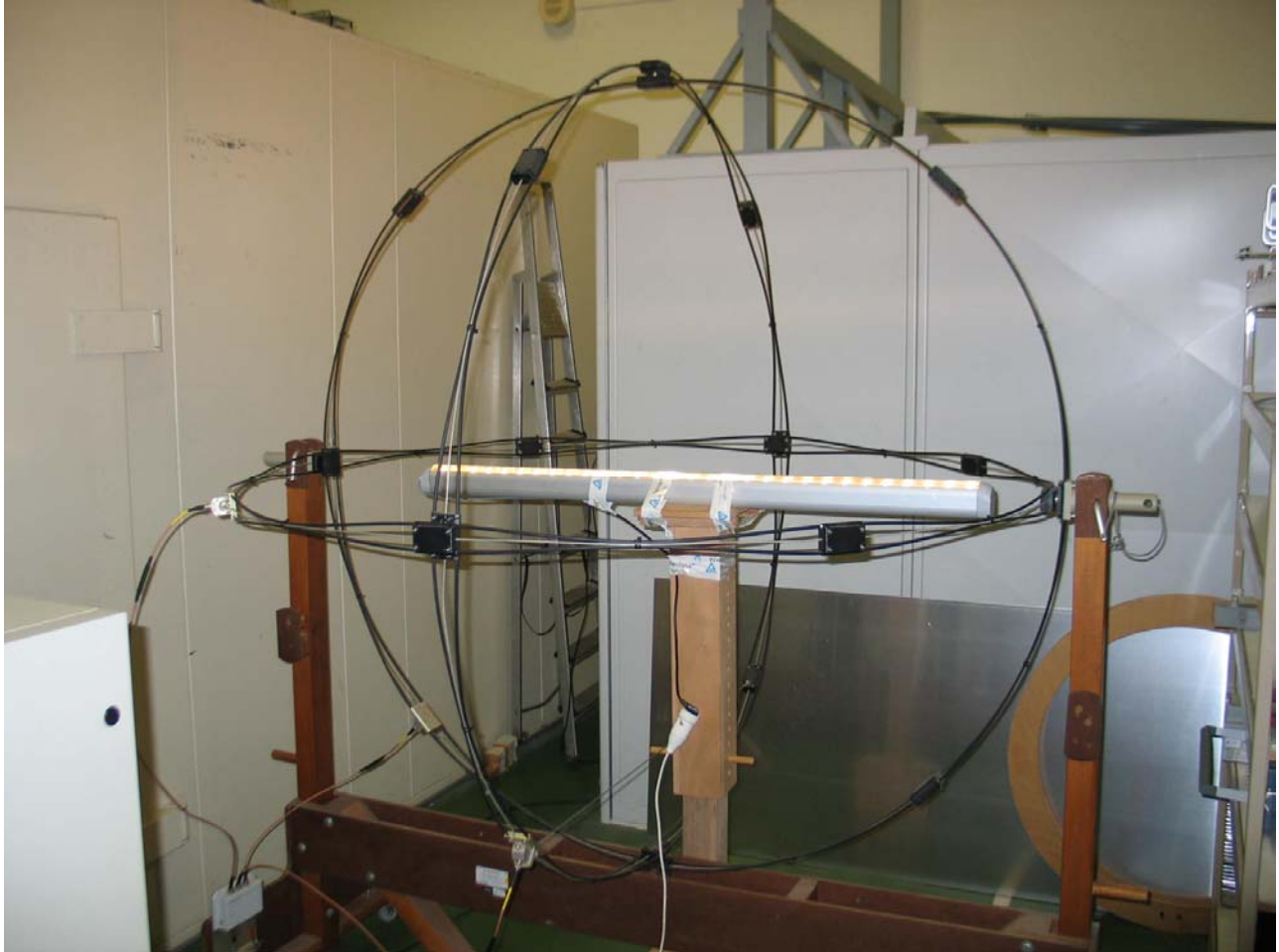
Photo 5 EUT during the magnetic emission test.
