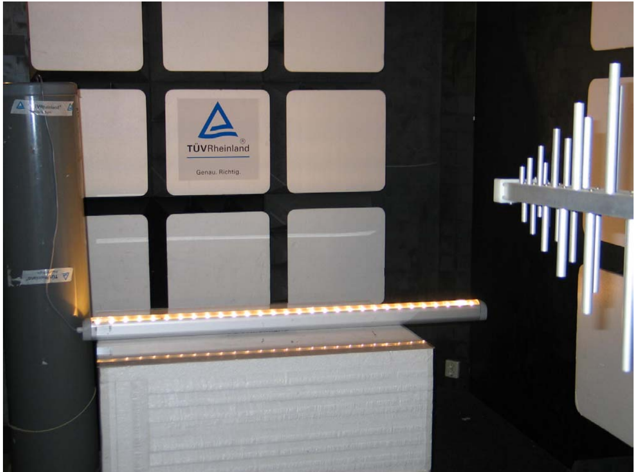
Photo 4. Set-up RF Radiated Immunity
