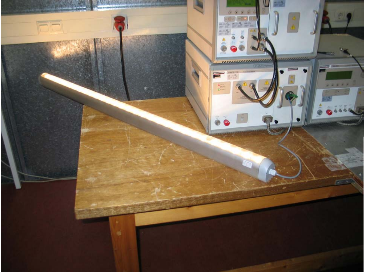
Photo 6. EUT during the surge test.
