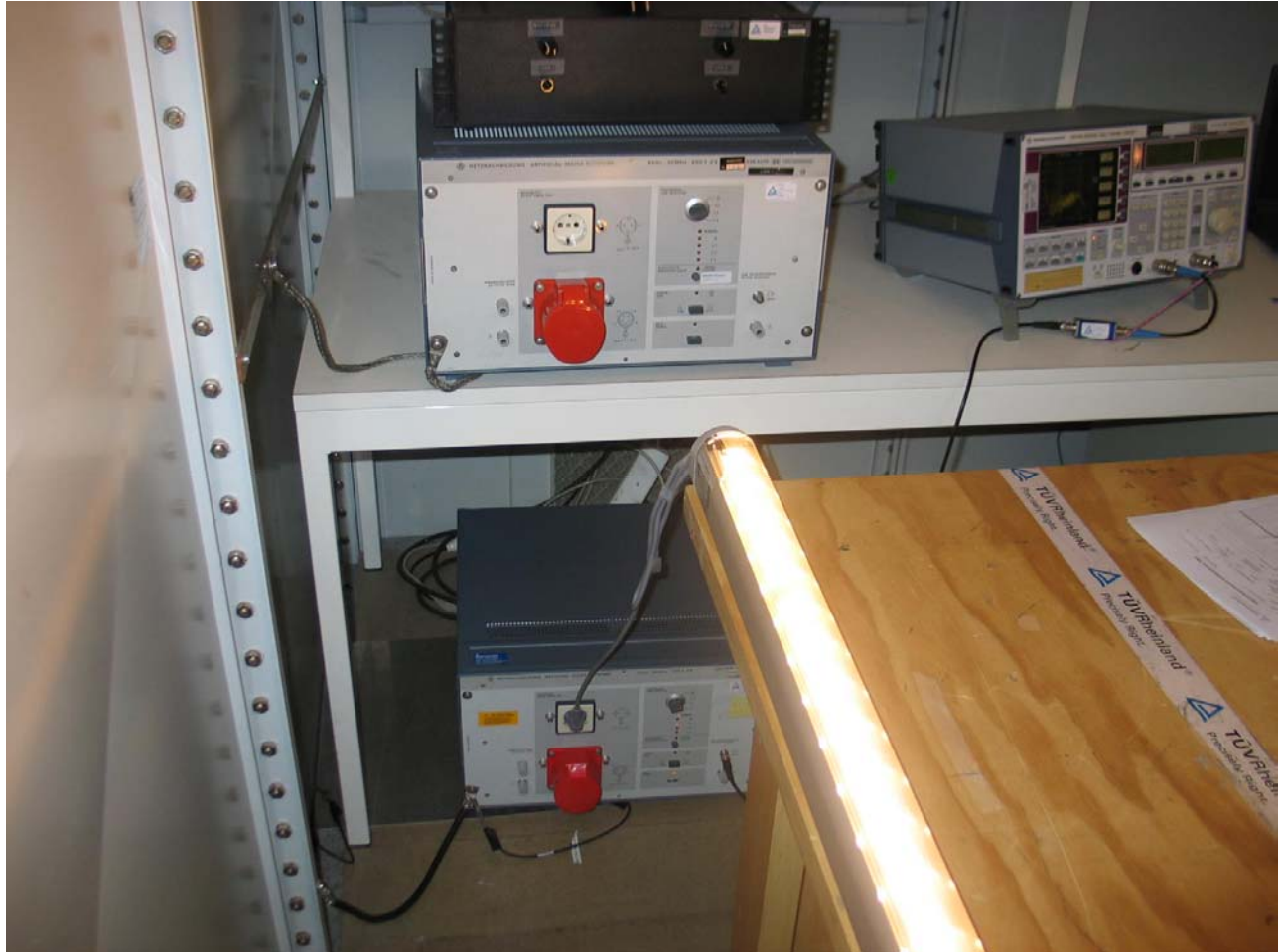
Photo 2. Test set-up during conducted emission tests
